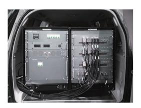
DRS-BL003 Reactive Convoy Jammer is specifically designed for protection of VIPs, convoys and high security premises against threats from possible terrorist acts of explosive devices through radio controlled detonation.
